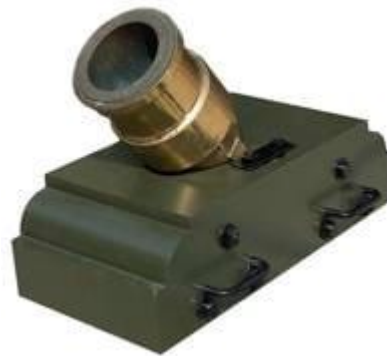
U.S. 24-pounder Coehorn mortar manufactured by Ames. No. 56, dated 1863.
