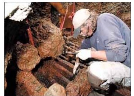
Jeff Johnston, historian of the Monitor National Marine Sanctuary, chisels concreted sediment from the roof of the turret. Joe Fudae/Dailv Press photo.
