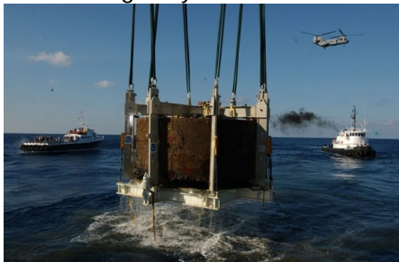
A team of conservators and researchers raises the turret of the USS Monitor out of the ocean on Aug. 5, 2002. (NOAA)
