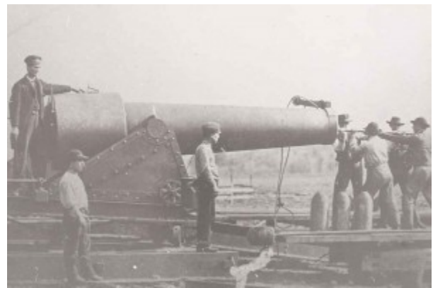
A crew loads a 300-pounder Parrott rifle that has been mounted on rails during the proofing process. (Paulson Brothers Ordnance Corp. Archive)
